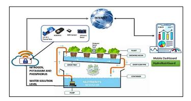
**Figure 2**. *HydroNutriGuard Technical Framework*
